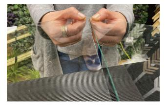
WHILE THERE ARE OTHER WAYS OF SNAPPING GLASS, THE METHOD OUTLINED BELOW IS MORE CONTROLLED AND THEREFORE A SAFE APPROACH WHEN STARTING TO WORK WITH GLASS.
