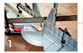
SAW HANDLE TO THE LEFT, SET @ 45°. MOULDING FED THROUGH FROM LEFT AND CLAMPED. SAW THE END.
