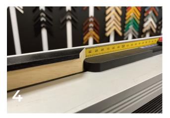
SET THE MITRED END UP AGAINST THE MITRE STOP. DON'T FORCE THE CONTACT. SOME OF THE MITRE SLIPS BEHIND THE "NOSE OF THE STOP.
