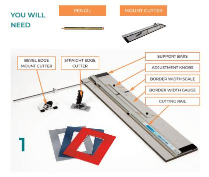
This describes the basic processes involved in cutting a simple window mount, using a Logan 350 Compact elite cutting system.
