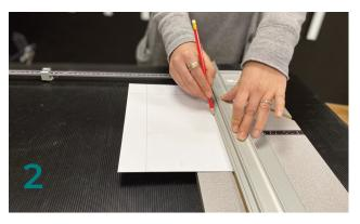
IDEA: When drawing in lines, ensure the pencil runs in at 45° to the rail so that the pencil "lead" runs along the rail edge.
